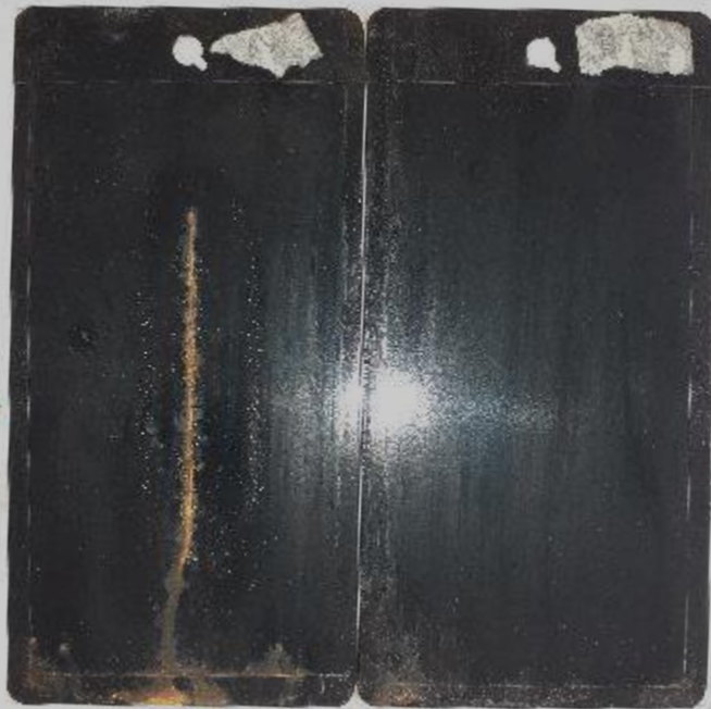
U-POL Engine Enamel 5 days salt spray Left panel scored
