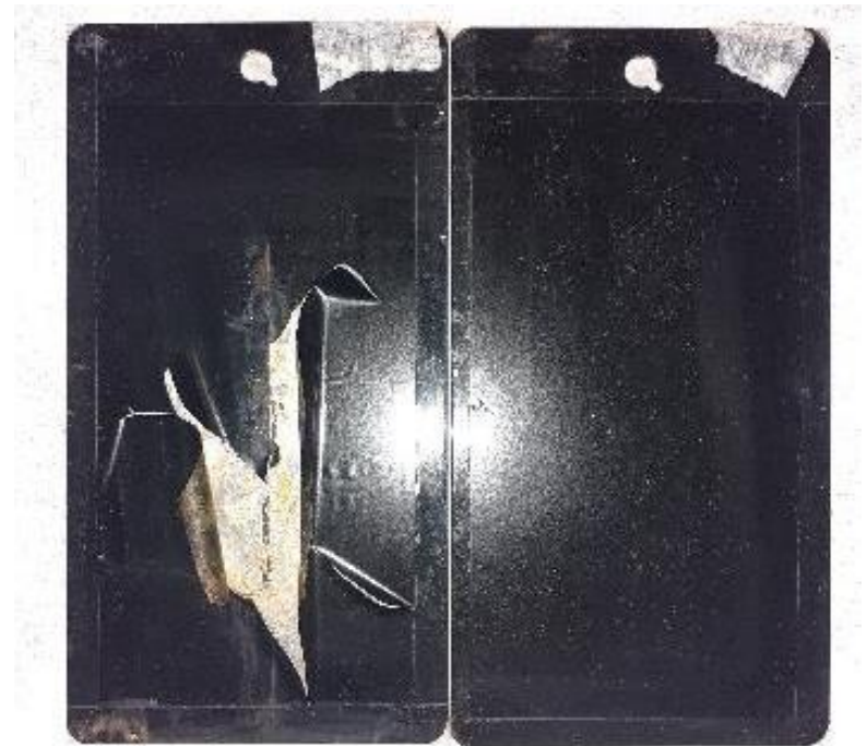
Competitor Engine Enamel 5 days salt spray Left panel scored
